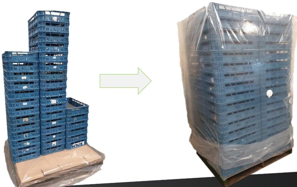
After the hermetic closure of the pallet cover, the vQm unit (connected to a CO2 gas bottle), is activated to suck residual air (to create a slight under pressure) and inject CO2. This cycle is repeated twice, and creates a high CO2 concentration (>35%) in the most efficient way possible.
